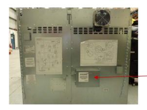
TO REMOVE REAR SERVICE PANELS REMOVE ALL SCREWS 12 X RIGHT HAND SIDE 12X LEFT HAND SIDE
