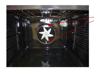
REMOVE THE 2 ELEMENT SECURING SCREWS AND PULL ELEMENT FORWARD INTO THE CAVITY
