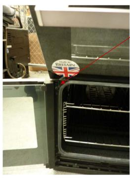
REMOVE THE 2 TOP HINGE SECURING SCREWS
