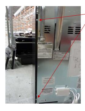
REMOVE 2X SCREWS AT REAR OF APPLIANCE
