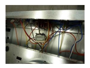
THE THERMOSTATS CAN NOW BE REMOVED BY PULLING OUT OF THE SWITCHPACK
