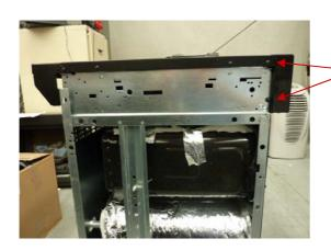
REMOVE 2 X SCREWS FROM EACH SIDE OF THE FACIA PANEL
